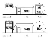
Examples of Sign Structure Area Measurements
